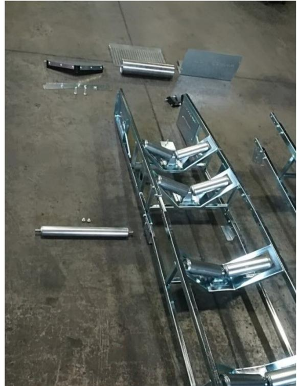
5 – Mount the intermediate frame with the tension frame and tighten the joints firmly
