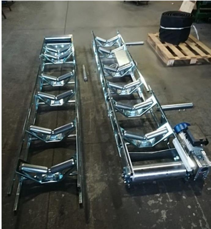
2 – Mount the intermediate frame with the control frame,
