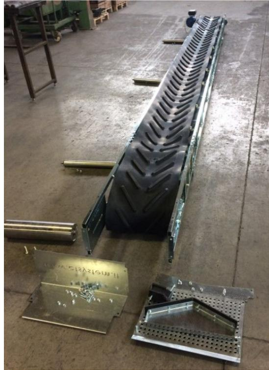
8 – Refit the tension cylinder, the return rollers and the tension plates.
