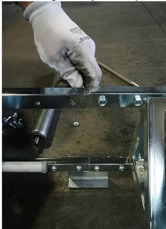
4 – Take the tension frame and disassemble the tension cylinder, the tension plates, the scraper and the return roller
